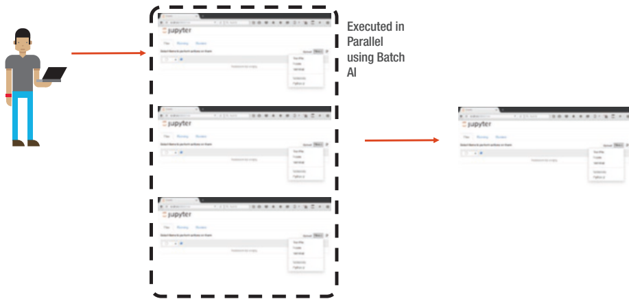
Figure 9-8. Rather than having to run Jupyter Notebooks in sequence to test different options, they can be executed in parallel using Batch AI
